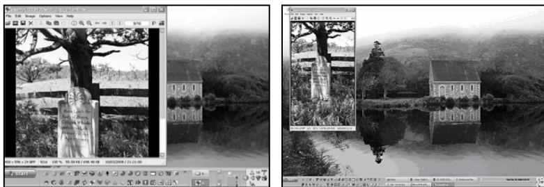
The same image shown at 100% on a screen set at 800x600 pixels (left) and then on a screen set at 1680x1050 pixels (right).
